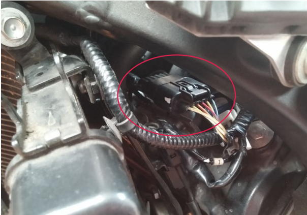
Pic.1 - location of 6way connector from Ignition coils
